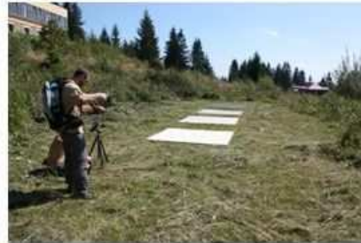
Artificial reference targets painted by Nextel Suede Coating
