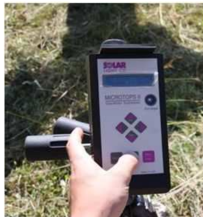
Actual state of atmosphere is estimated from Microtops II measurements
