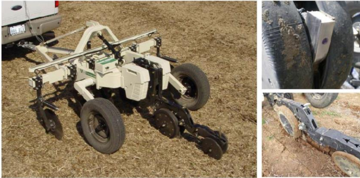
Figure 1. Veris OpticMapper with Soil EC and Optical Sensors.
